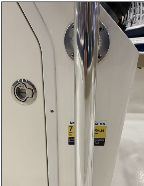
Incorrect Capacity Plate Placement- side of center console and obscured.
