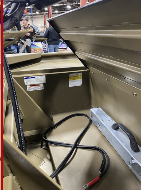
Here it is ... incorrect Capacity Plate Placement - only visible with hatch open
