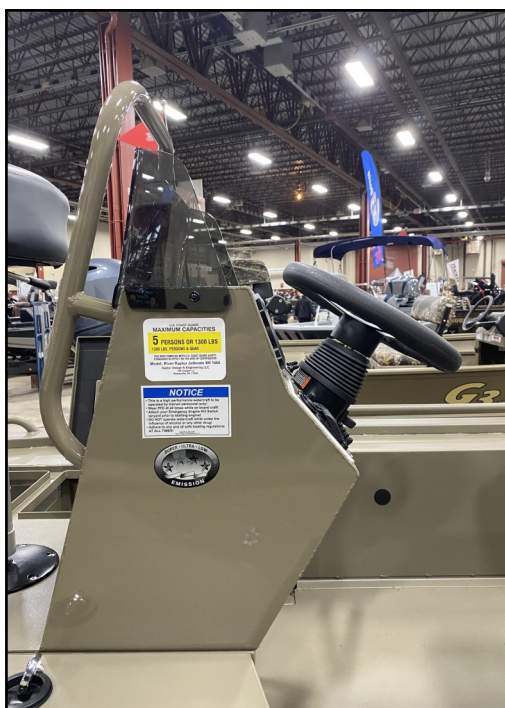
Incorrect Capacity Plate - side of center console and out of the operator's line of sight.
