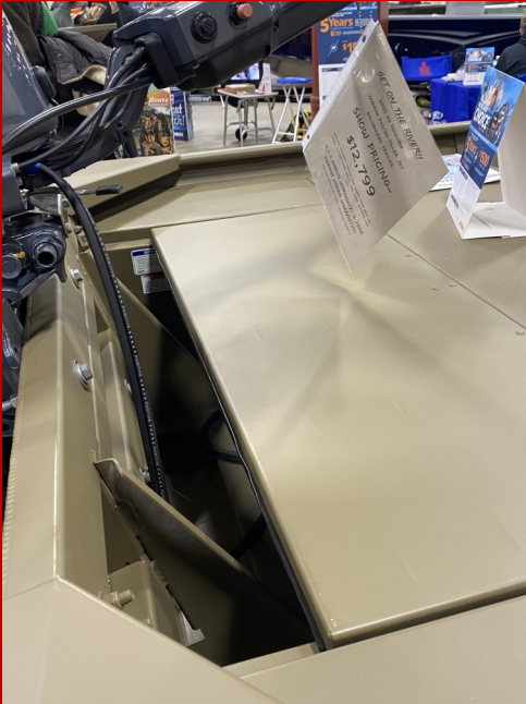
Where is the Capacity Label ... incorrect Capacity Plate Placement— hatch closed, hidden.
